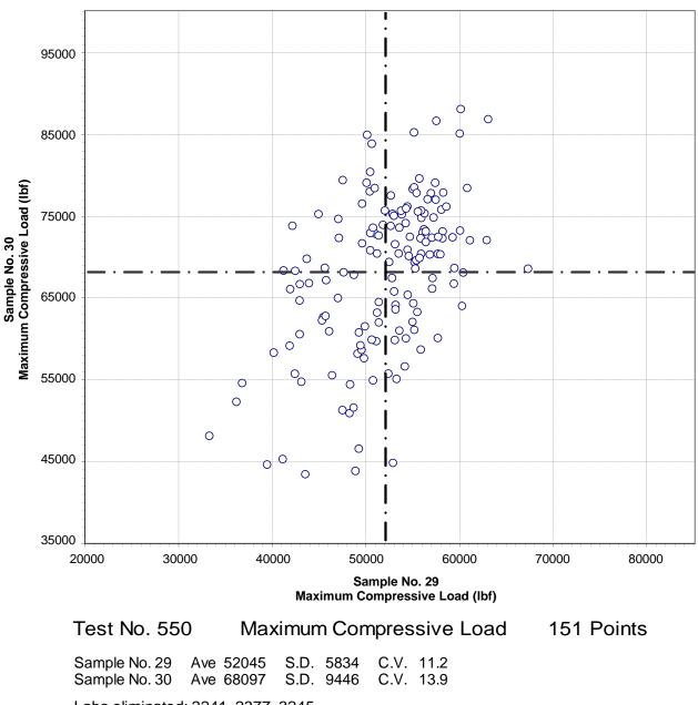
CCRL Proficiency Sample Program Maximum Compressive Load CONCRETE MASONRY UNITS Samples No. 29 and No. 30
