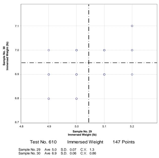
CCRL Proficiency Sample Program Immersed Weight CONCRETE MASONRY UNITS Samples No. 29 and No. 30
