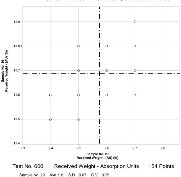
CCRL Proficiency Sample Program Received Weight - Absorption Units CONCRETE MASONRY UNITS Samples No. 29 and No. 30
