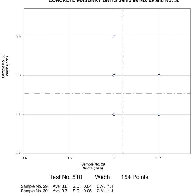
CCRL Proficiency Sample Program Width CONCRETE MASONRY UNITS Samples No. 29 and No. 30
