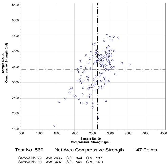
CCRL Proficiency Sample Program Net Area Compressive Strength CONCRETE MASONRY UNITS Samples No. 29 and No. 30
