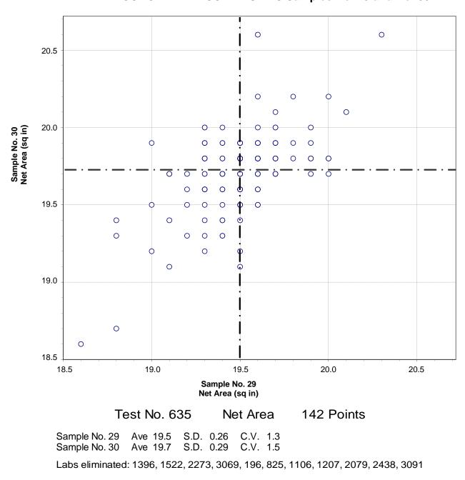
CCRL Proficiency Sample Program Net Area CONCRETE MASONRY UNITS Samples No. 29 and No. 30
