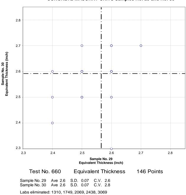
CCRL Proficiency Sample Program Equivalent Thickness CONCRETE MASONRY UNITS Samples No. 29 and No. 30
