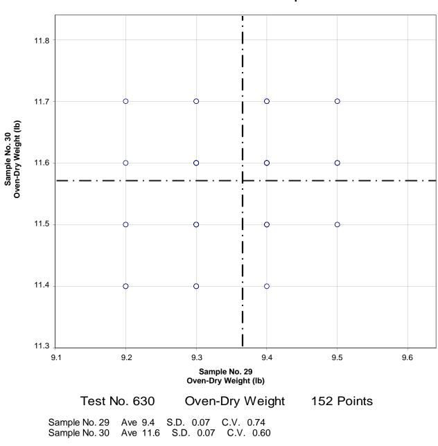
CCRL Proficiency Sample Program Oven-Dry Weight CONCRETE MASONRY UNITS Samples No. 29 and No. 30
