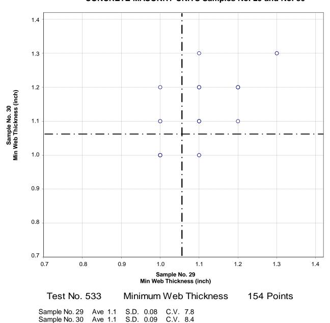
CCRL Proficiency Sample Program Minimum Web Thickness CONCRETE MASONRY UNITS Samples No. 29 and No. 30
