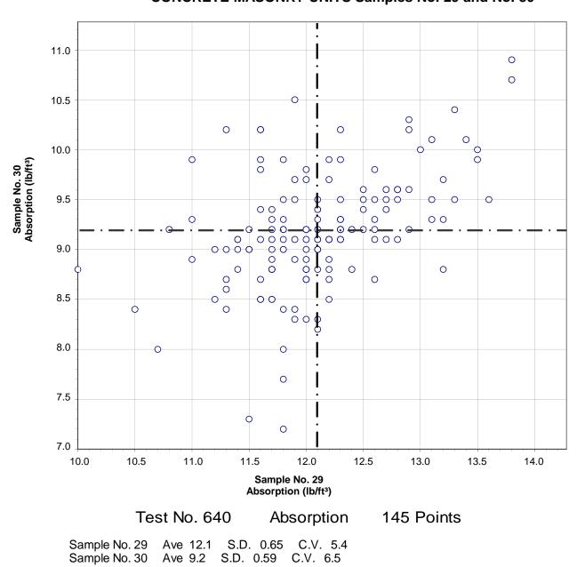
CCRL Proficiency Sample Program Absorption CONCRETE MASONRY UNITS Samples No. 29 and No. 30
