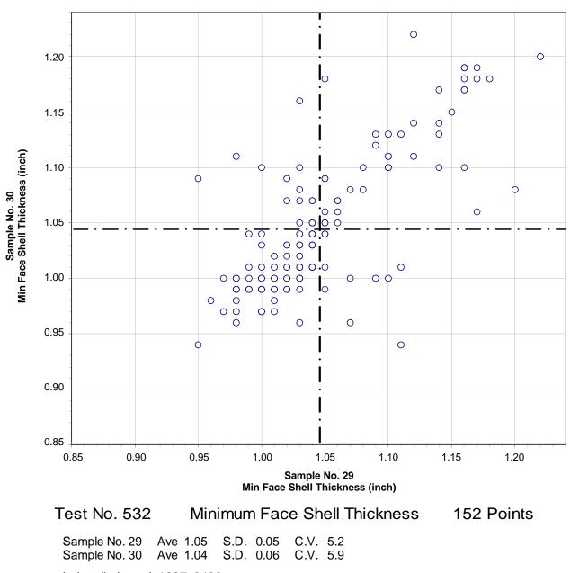
CCRL Proficiency Sample Program Minimum Face Shell Thickness CONCRETE MASONRY UNITS Samples No. 29 and No. 30
