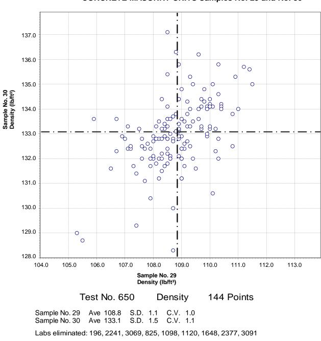
CCRL Proficiency Sample Program Density CONCRETE MASONRY UNITS Samples No. 29 and No. 30
