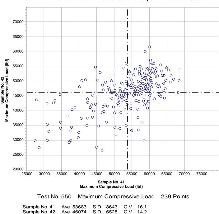
CCRL Proficiency Sample Program Maximum Compressive Load CONCRETE MASONRY UNITS Samples No. 41 and No. 42
