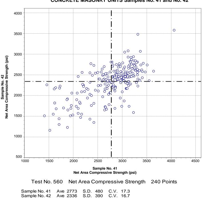
Net Area Compressive Strength CONCRETE MASONRY UNITS Samples No. 41 and No. 42
