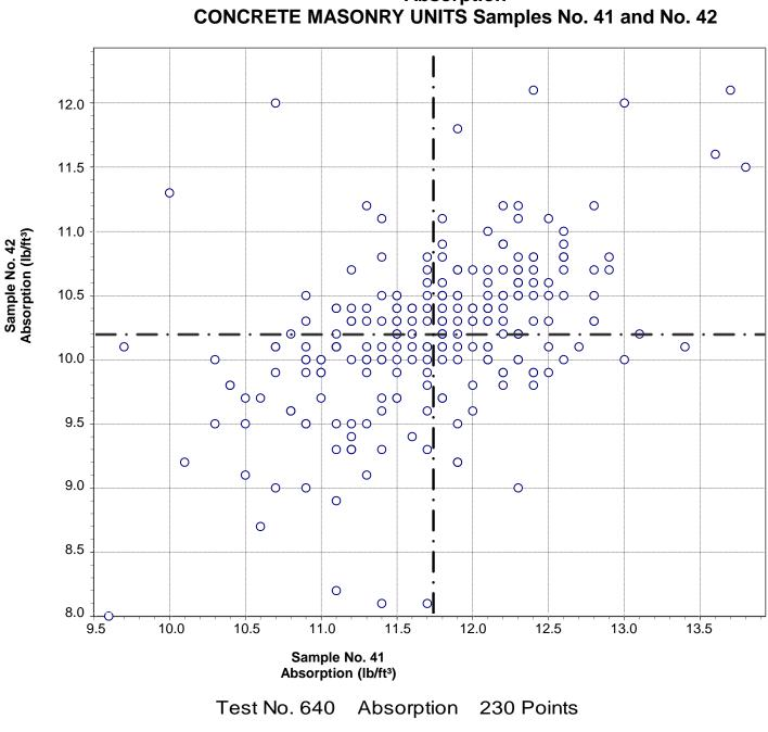
CCRL Proficiency Sample Program Absorption CONCRETE MASONRY UNITS Samples No. 41 and No. 42
