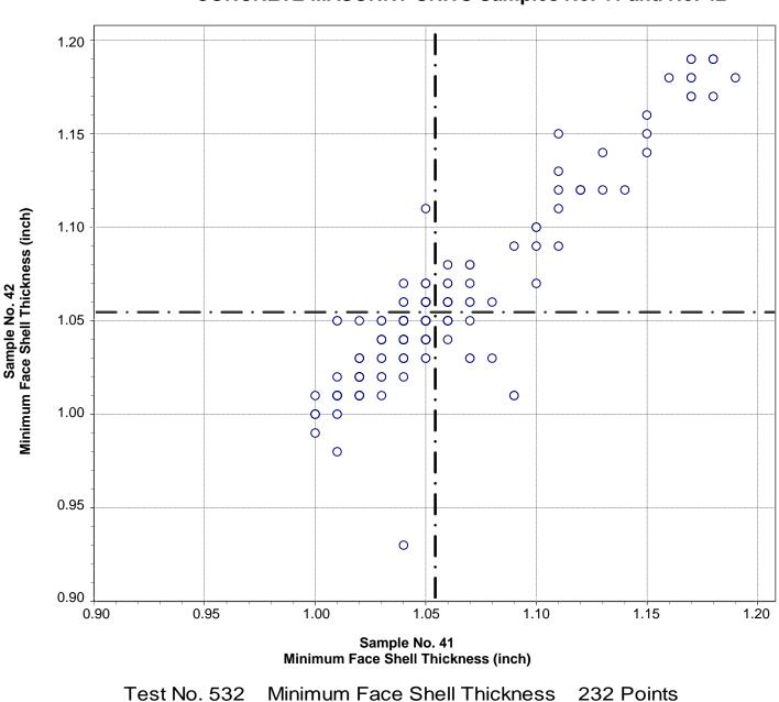
CCRL Proficiency Sample Program Minimum Face Shell Thickness CONCRETE MASONRY UNITS Samples No. 41 and No. 42
