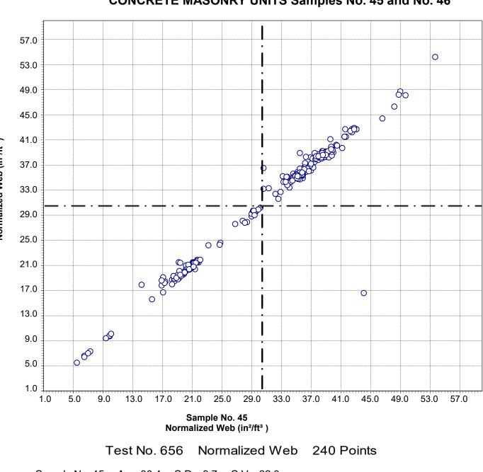
CCRL Proficiency Sample Program Normalized Web CONCRETE MASONRY UNITS Samples No. 45 and No. 46
