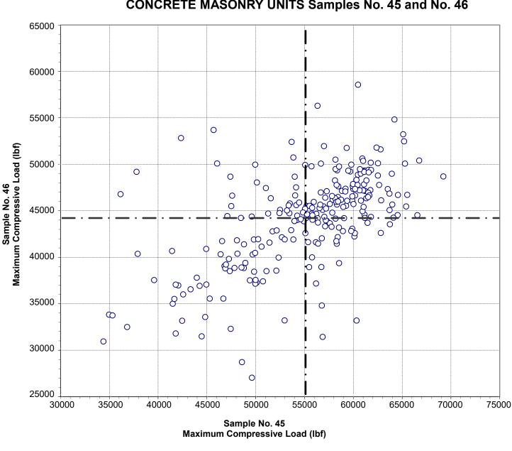
CCRL Proficiency Sample Program Maximum Compressive Load CONCRETE MASONRY UNITS Samples No. 45 and No. 46
