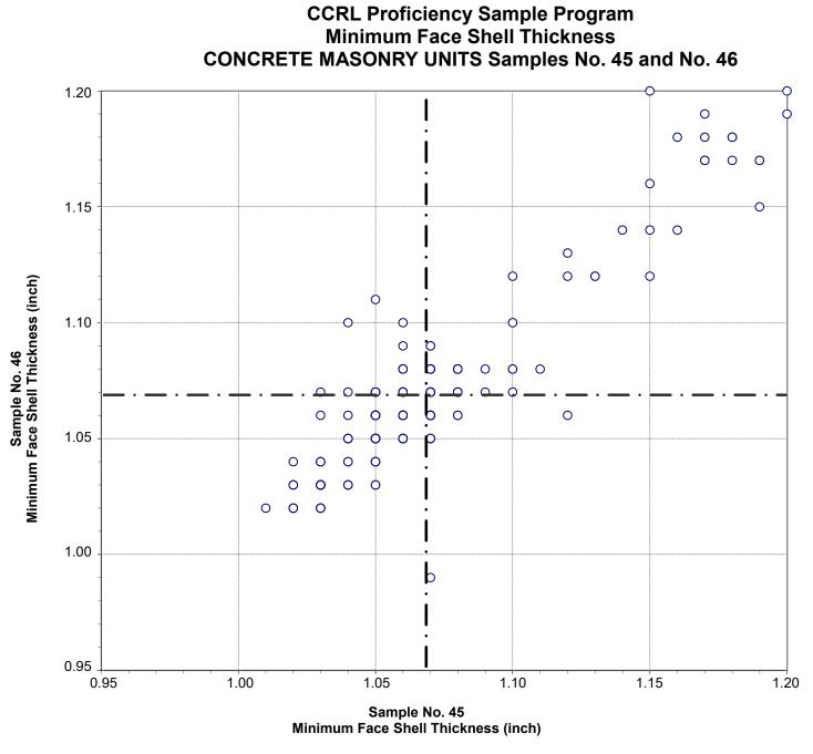
Test No. 532 Minimum Face Shell Thickness 244 Points
