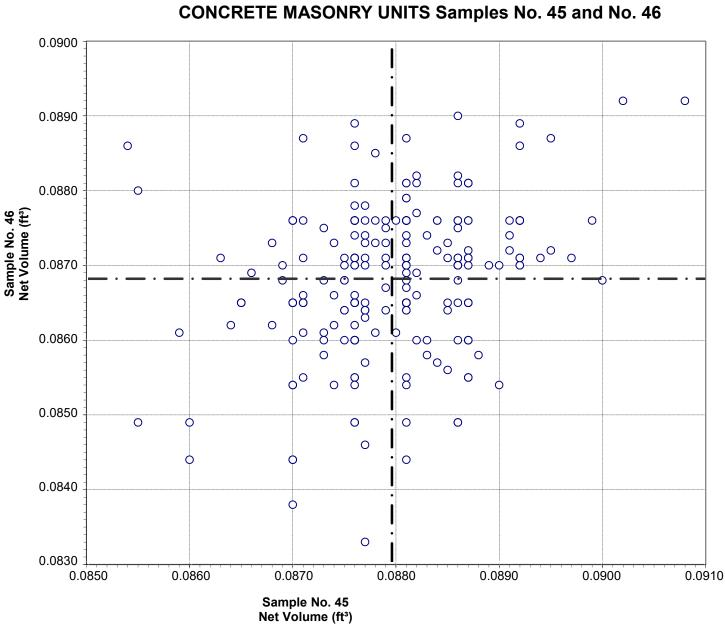
CCRL Proficiency Sample Program Net Volume CONCRETE MASONRY UNITS Samples No. 45 and No. 46
