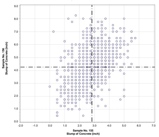
Test No. 2 Slump of Concrete 1233 Points
