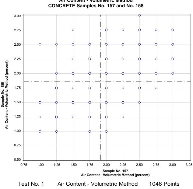
CCRL Proficiency Sample Program Air Content - Volumetric Method CONCRETE Samples No. 157 and No. 158
