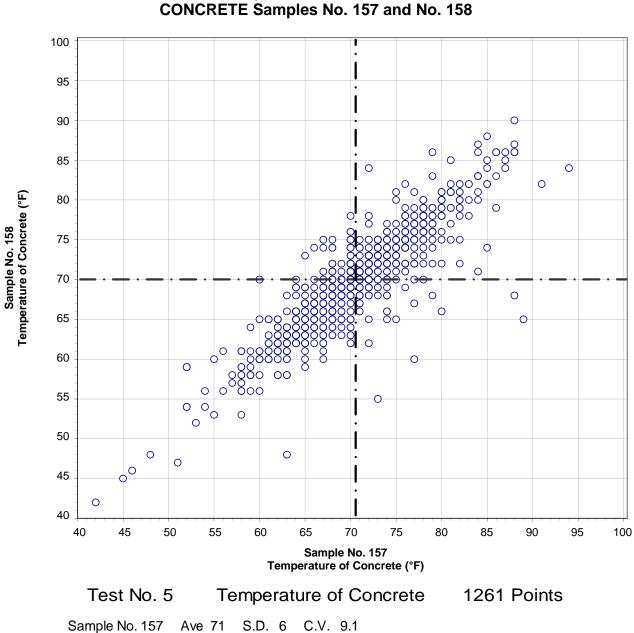
CCRL Proficiency Sample Program Temperature of Concrete CONCRETE Samples No. 157 and No. 158
