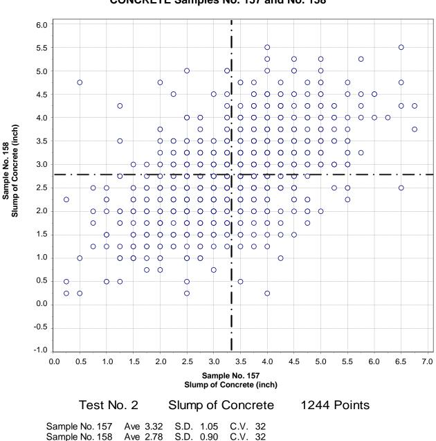
CCRL Proficiency Sample Program Slump of Concrete CONCRETE Samples No. 157 and No. 158
