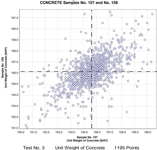
CCRL Proficiency Sample Program Unit Weight of Concrete CONCRETE Samples No. 157 and No. 157
