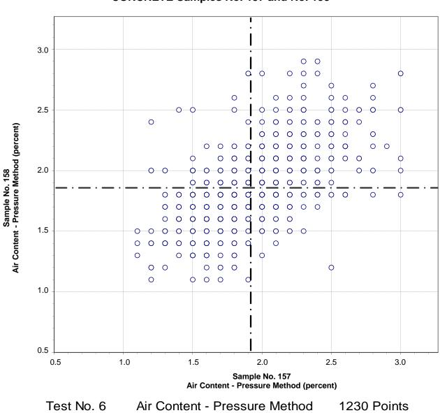
CCRL Proficiency Sample Program Air Content - Pressure Method CONCRETE Samples No. 157 and No. 158
