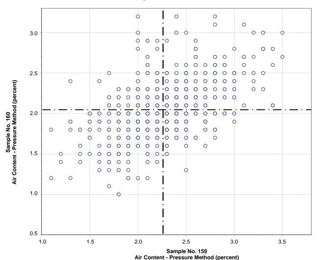
Test No. 6 Air Content - Pressure Method 1242 Points
