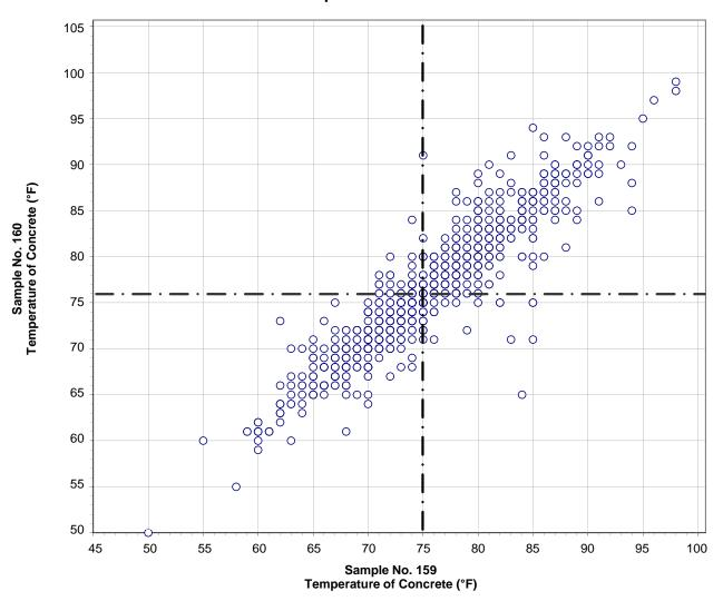
Test No. 5 Temperature of Concrete 1277 Points
