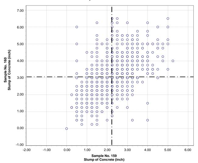
Test No. 2 Slump of Concrete 1255 Points
