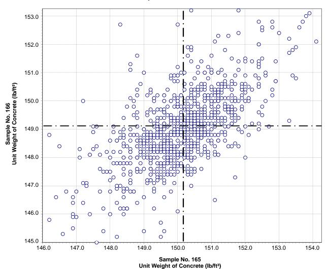
Test No. 3 Unit Weight of Concrete 1276 Points
