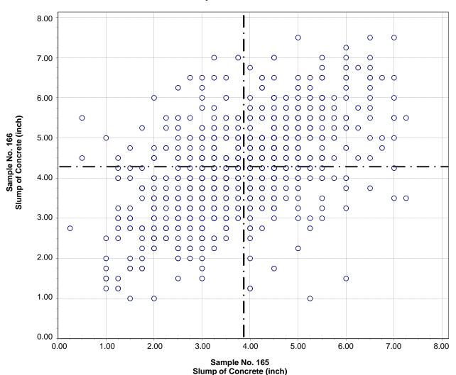
Test No. 2 Slump of Concrete 1316 Points
