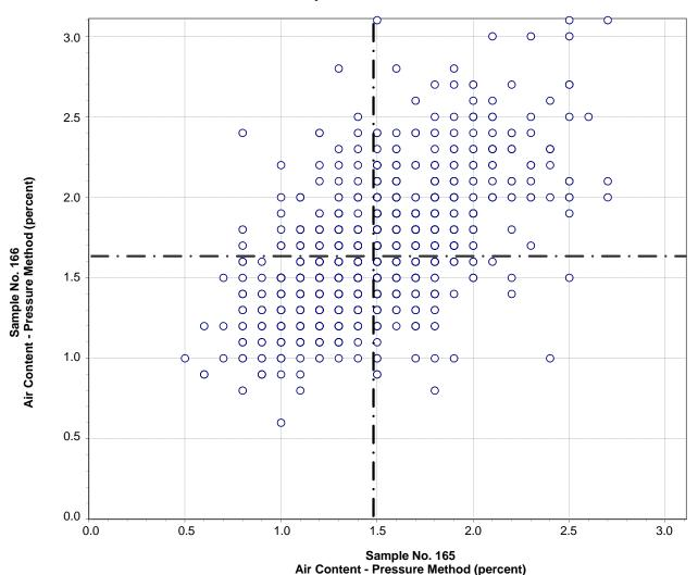
Test No. 6 Air Content - Pressure Method 1301 Points
