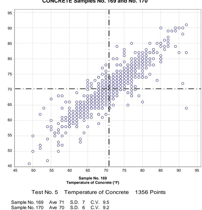
Temperature of Concrete CONCRETE Samples No. 169 and No. 170
