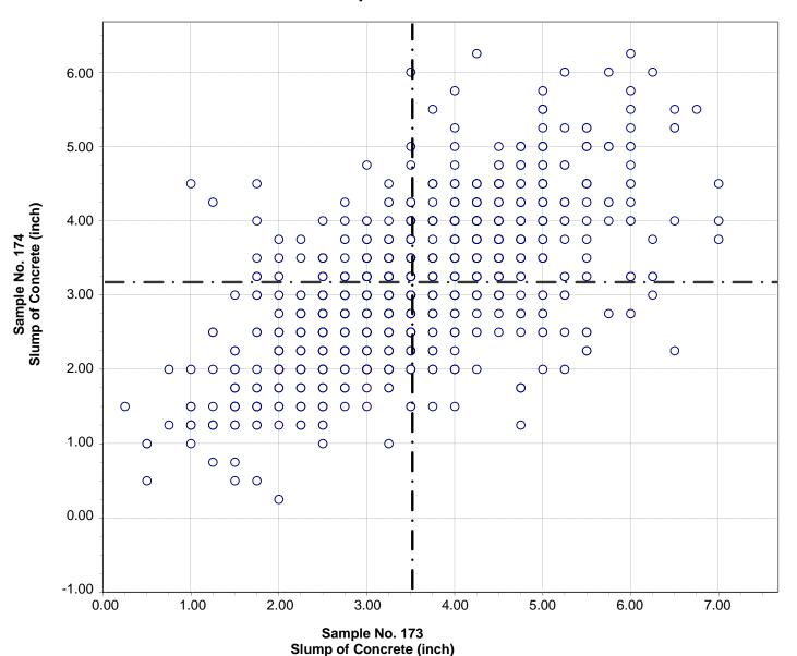
Test No. 2 Slump of Concrete 1399 Points
