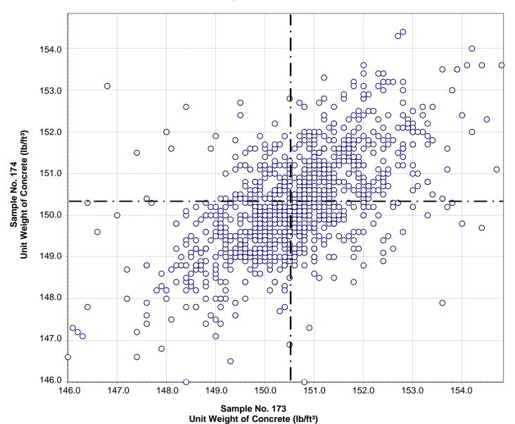
Test No. 3 Unit Weight of Concrete 1358 Points
