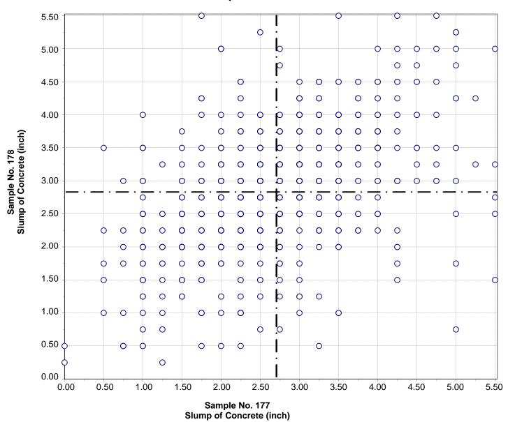
Test No. 2 Slump of Concrete 1428 Points
