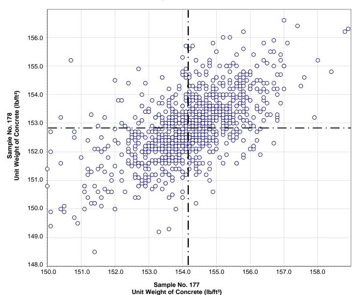
Test No. 3 Unit Weight of Concrete 1377 Points
