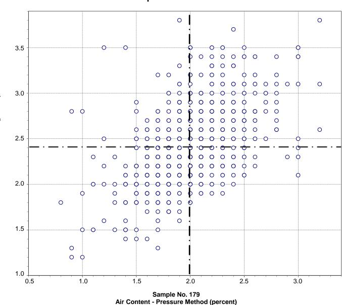
CCRL Proficiency Sample Program Air Content - Pressure Method CONCRETE Samples No. 179 and No. 180
