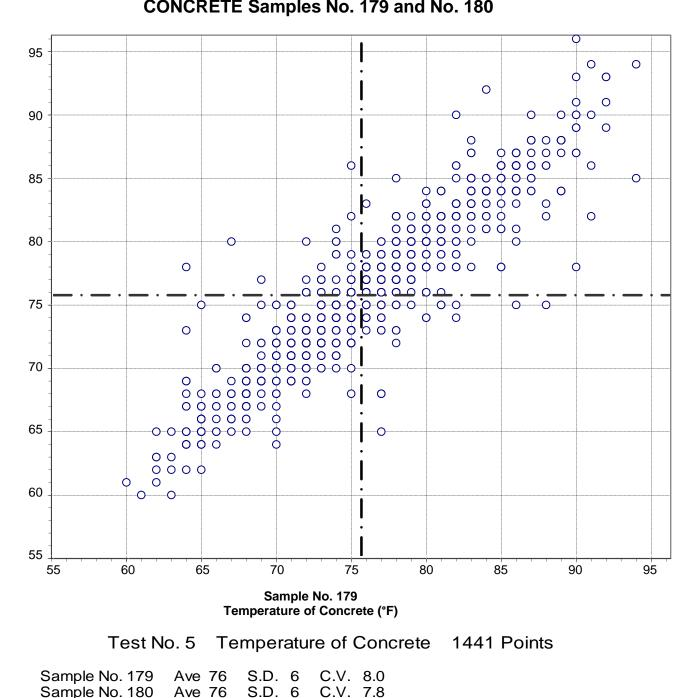
CCRL Proficiency Sample Program Temperature of Concrete CONCRETE Samples No. 179 and No. 180
