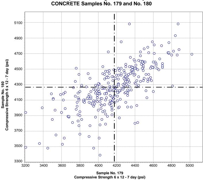
CCRL Proficiency Sample Program Compressive Strength 6 x 12 - 7 day CONCRETE Samples No. 179 and No. 180
