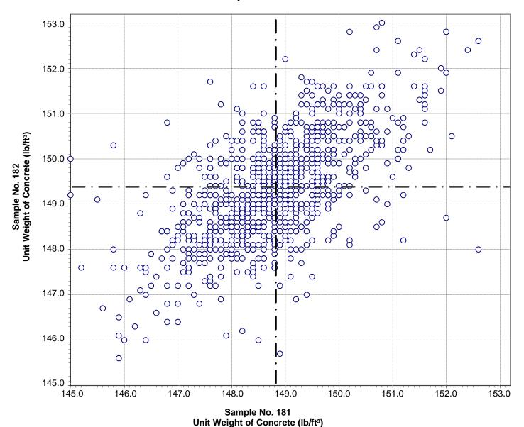
Test No. 3 Unit Weight of Concrete 1419 Points
