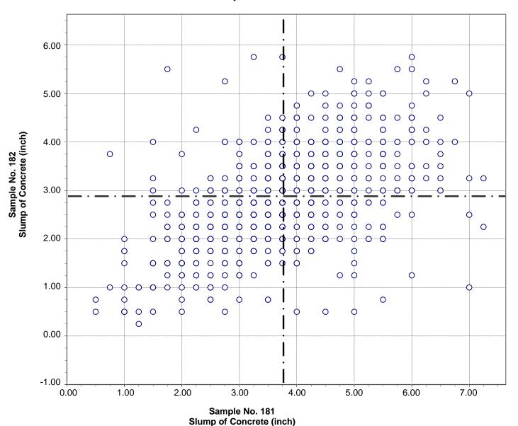
Test No. 2 Slump of Concrete 1456 Points
