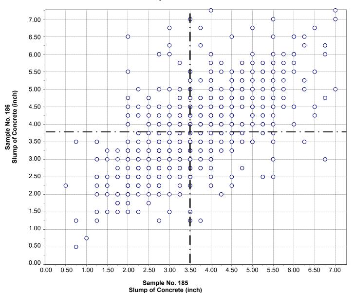
Test No. 2 Slump of Concrete 1449 Points
