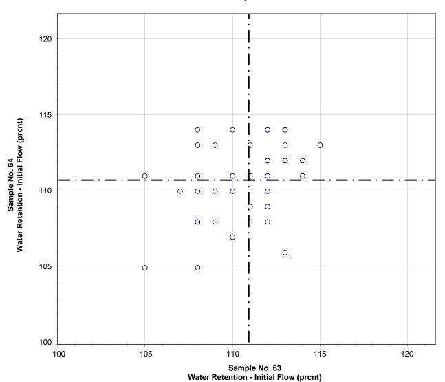
Test No. 331 Water Retention - Initial Flow 62 Points
