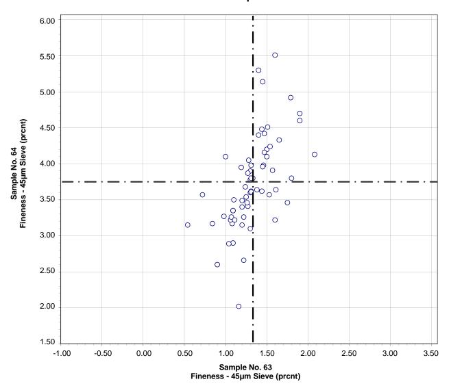
Test No. 281 Fineness - 45µm Sieve Retained 63 Points
