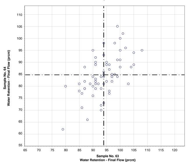
Test No. 332 Water Retention - Final Flow 63 Points
