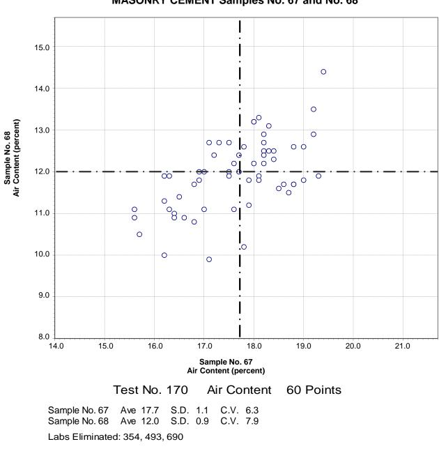
CCRL Proficiency Sample Program Air Content MASONRY CEMENT Samples No. 67 and No. 68
