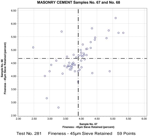
CCRL Proficiency Sample Program Fineness - 45µm Sieve Retained MASONRY CEMENT Samples No. 67 and No. 68
