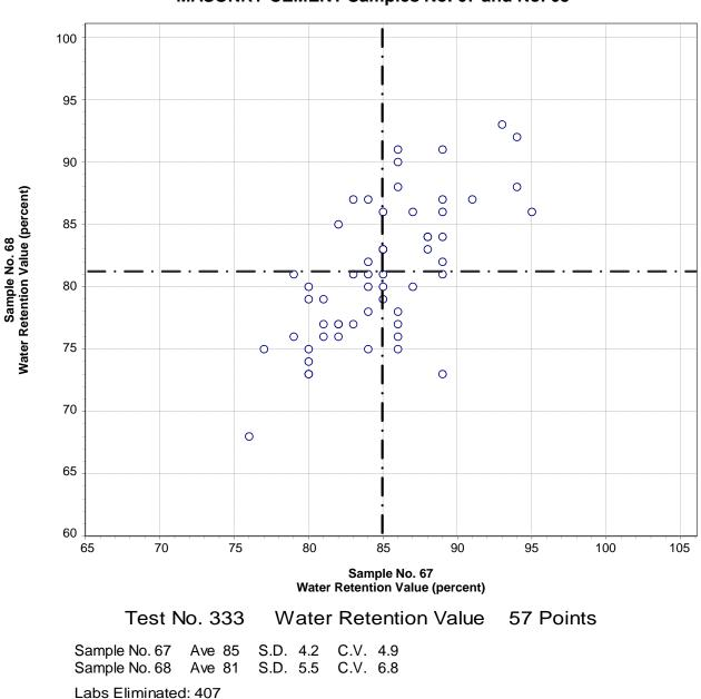
CCRL Proficiency Sample Program Water Retention Value MASONRY CEMENT Samples No. 67 and No. 68
