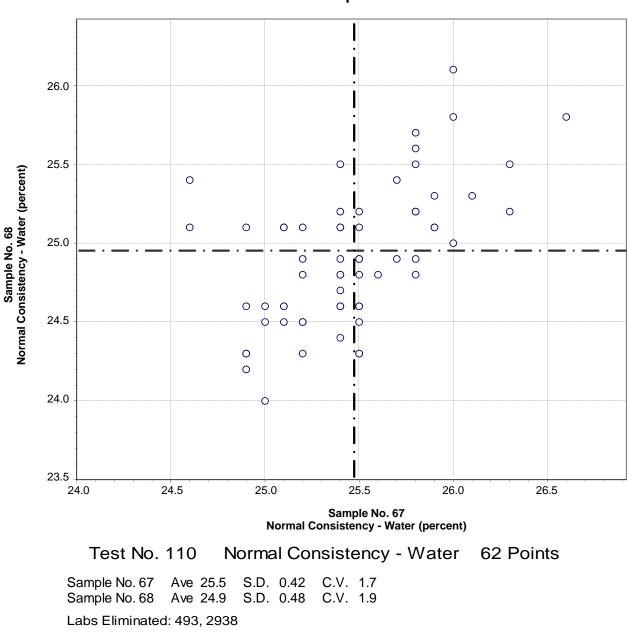
CCRL Proficiency Sample Program Normal Consistency - Water MASONRY CEMENT Samples No. 67 and No. 68
