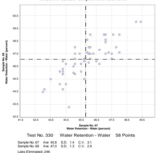
CCRL Proficiency Sample Program Water Retention - Water MASONRY CEMENT Samples No. 67 and No. 68
