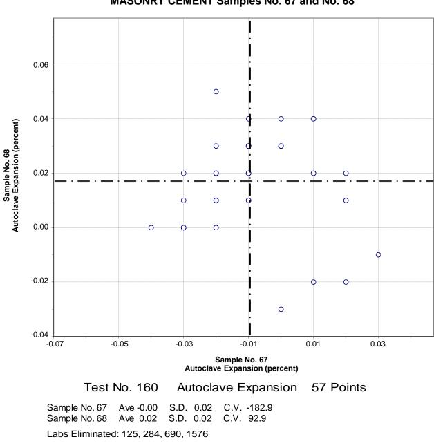
Autoclave Expansion MASONRY CEMENT Samples No. 67 and No. 68
