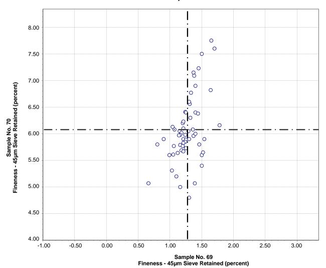
Test No. 281 Fineness - 45µm Sieve Retained 58 Points
