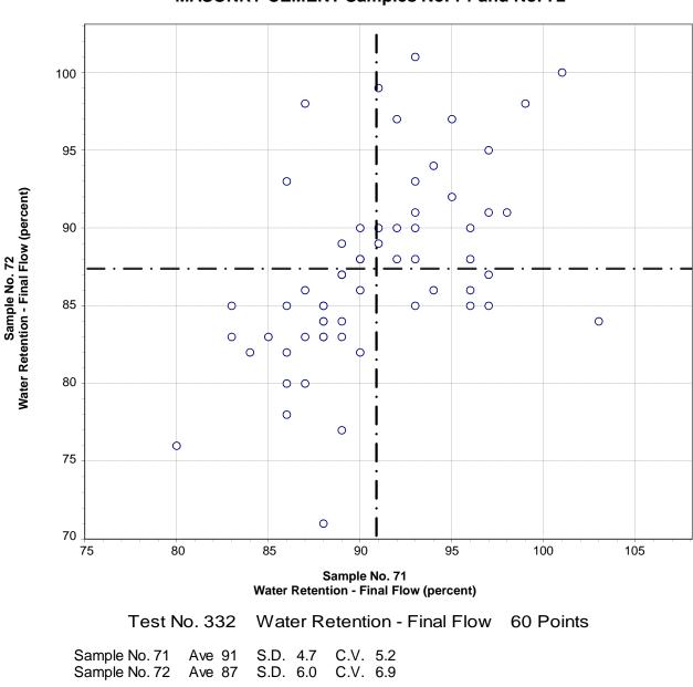
CCRL Proficiency Sample Program Water Retention - Final Flow MASONRY CEMENT Samples No. 71 and No. 72
