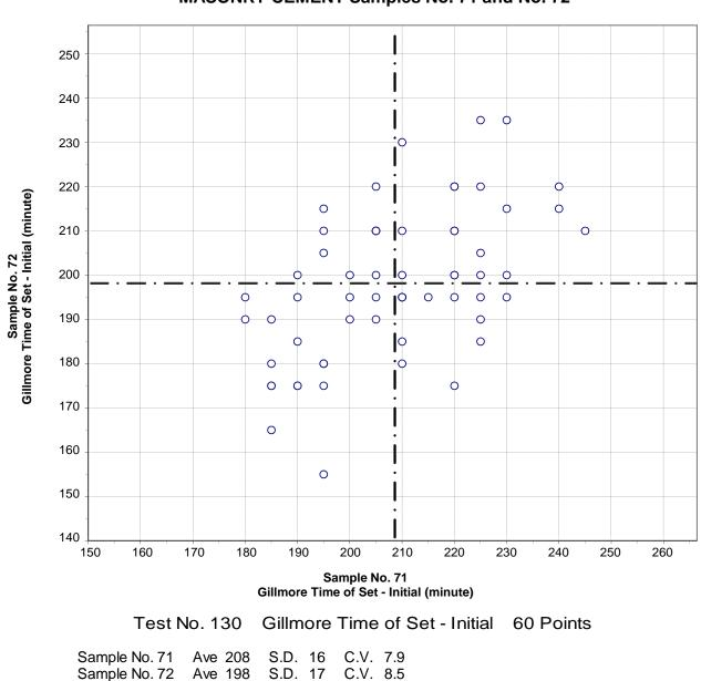
CCRL Proficiency Sample Program Gillmore Time of Set - Initial MASONRY CEMENT Samples No. 71 and No. 72
