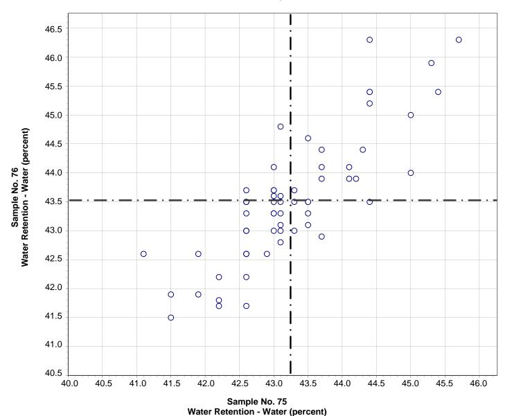
Test No. 330 Water Retention - Water 63 Points
