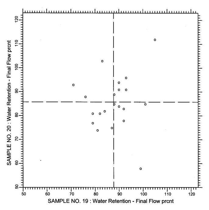
TEST NO.332 Water Retention - Final Flow 21 POINTS
