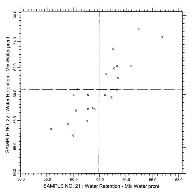
TEST NO.330 Water Retention - Mix Water
