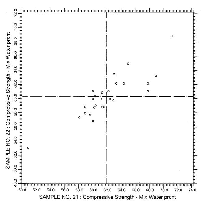
TEST NO.220 Compressive Strength - Mix Water 28 POINTS
