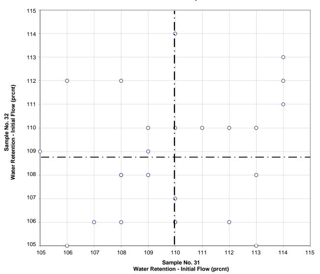
Test No. 331 Water Retention - Initial Flow 26 Points
