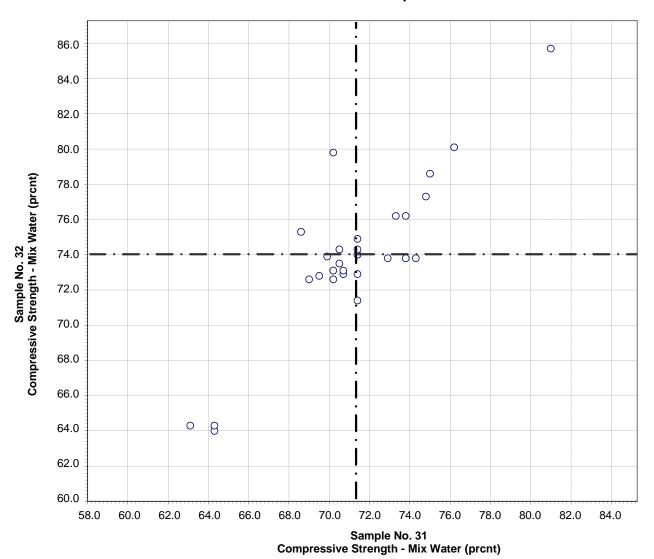
Test No. 220 Compressive Strength - Mix Water 30 Points
