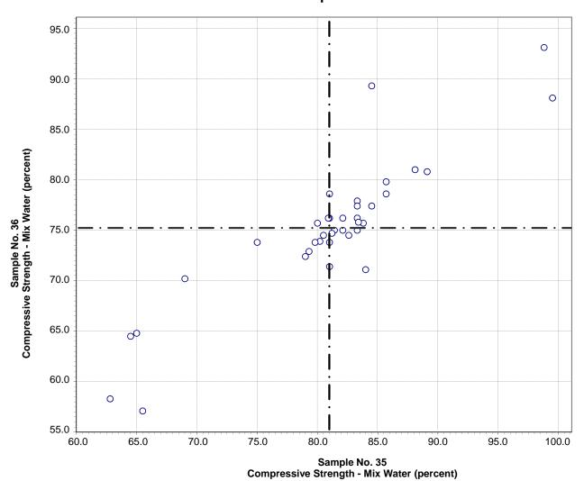
Test No. 220 Compressive Strength - Mix Water 37 Points
