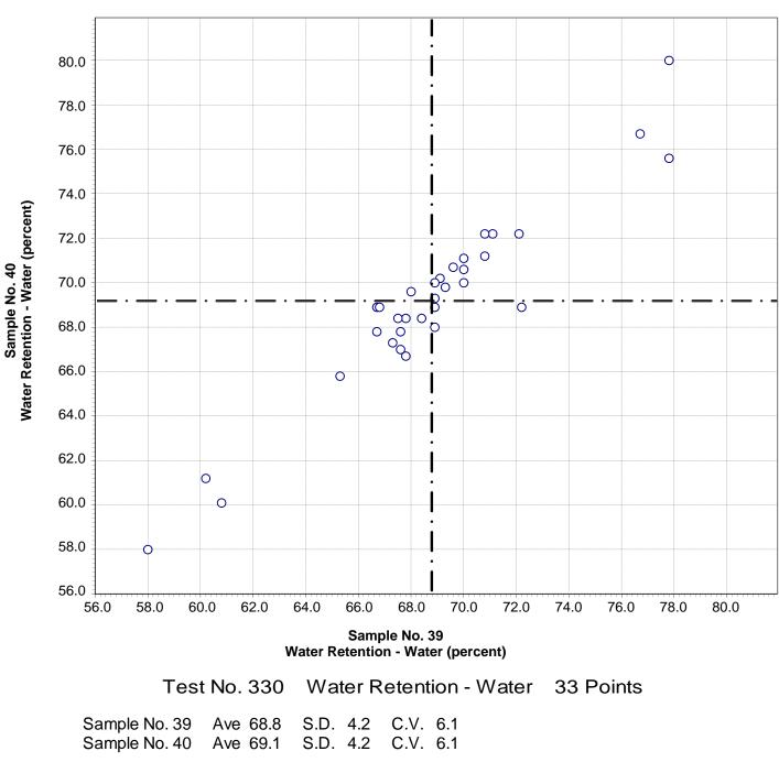
CCRL Proficiency Sample Program Water Retention - Water MASONRY MORTAR Samples No. 39 and No. 40
