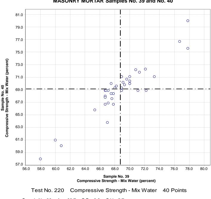
CCRL Proficiency Sample Program Compressive Strength - Mix Water MASONRY MORTAR Samples No. 39 and No. 40
