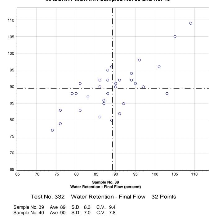
CCRL Proficiency Sample Program Water Retention - Final Flow MASONRY MORTAR Samples No. 39 and No. 40
