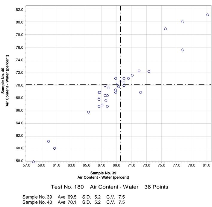
**CCRL Proficiency Sample Program** Air Content - Water **MASONRY MORTAR Samples No. 39 and No. 40**
