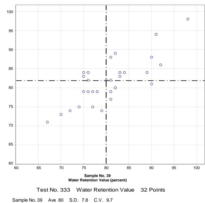
CCRL Proficiency Sample Program Water Retention Value MASONRY MORTAR Samples No. 39 and No. 40
