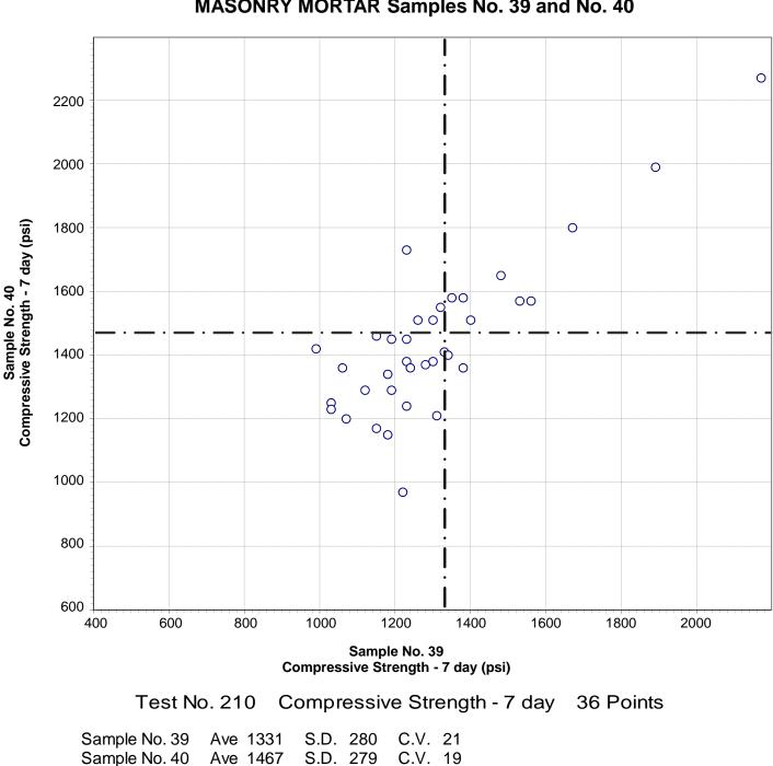
Compressive Strength - 7 day MASONRY MORTAR Samples No. 39 and No. 40
