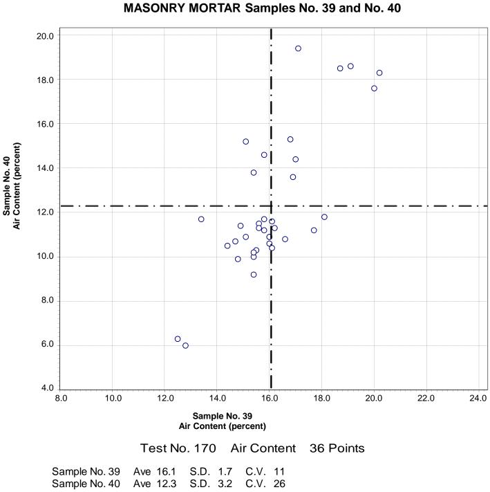
CCRL Proficiency Sample Program Air Content MASONRY MORTAR Samples No. 39 and No. 40
