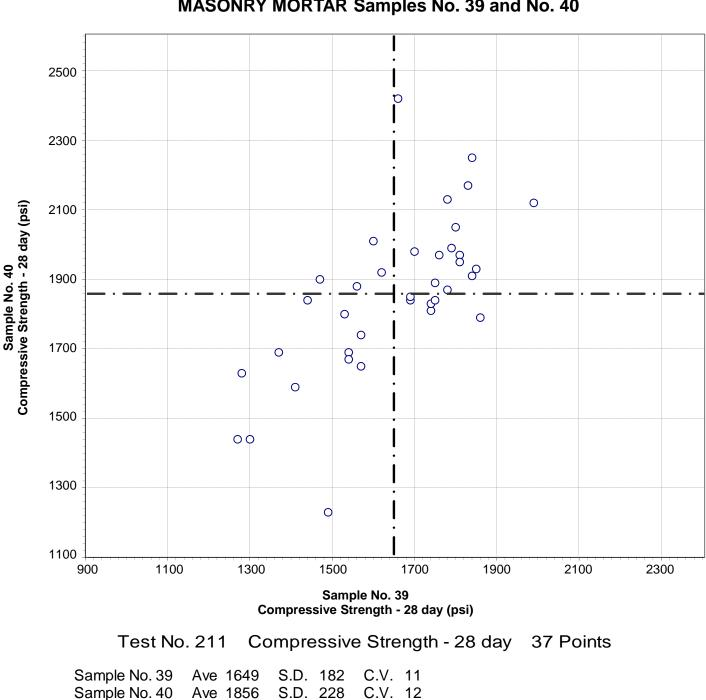
CCRL Proficiency Sample Program Compressive Strength - 28 day MASONRY MORTAR Samples No. 39 and No. 40
