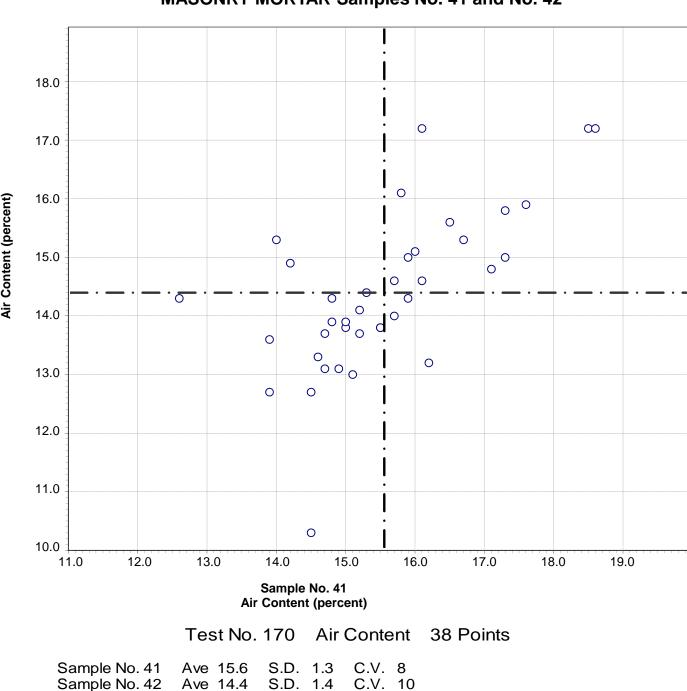
**CCRL Proficiency Sample Program** Air Content **MASONRY MORTAR Samples No. 41 and No. 42**
