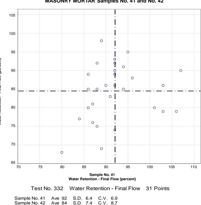
CCRL Proficiency Sample Program Water Retention - Final Flow MASONRY MORTAR Samples No. 41 and No. 42
