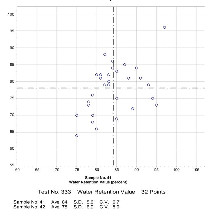
Water Retention Value MASONRY MORTAR Samples No. 41 and No. 42
