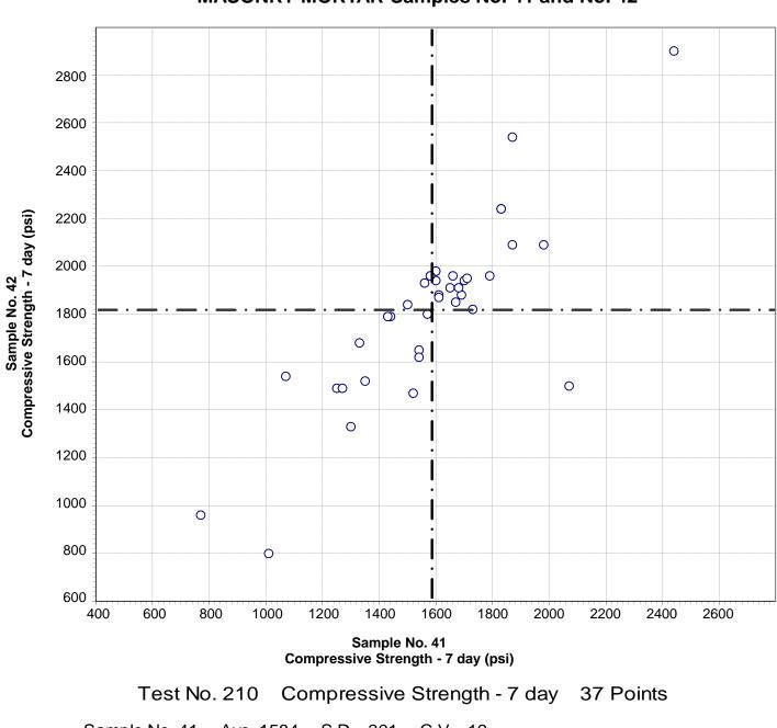
CCRL Proficiency Sample Program Compressive Strength - 7 day MASONRY MORTAR Samples No. 41 and No. 42
