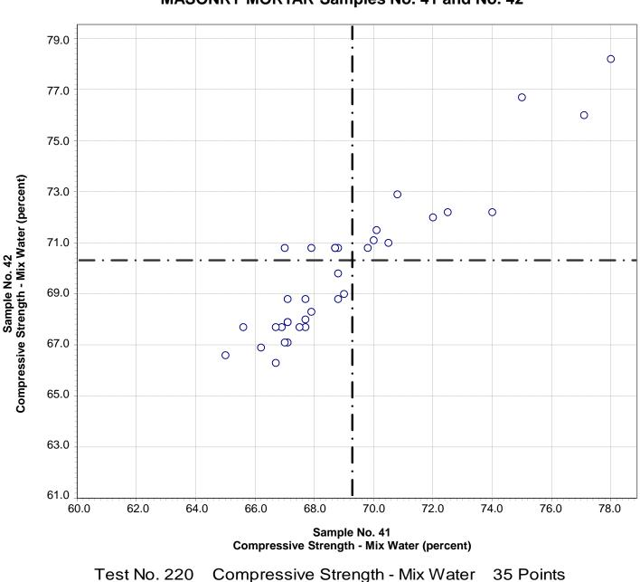
CCRL Proficiency Sample Program Compressive Strength - Mix Water MASONRY MORTAR Samples No. 41 and No. 42
