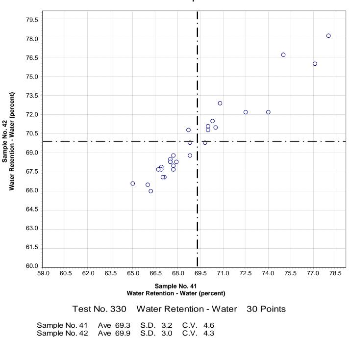
Water Retention - Water MASONRY MORTAR Samples No. 41 and No. 42
