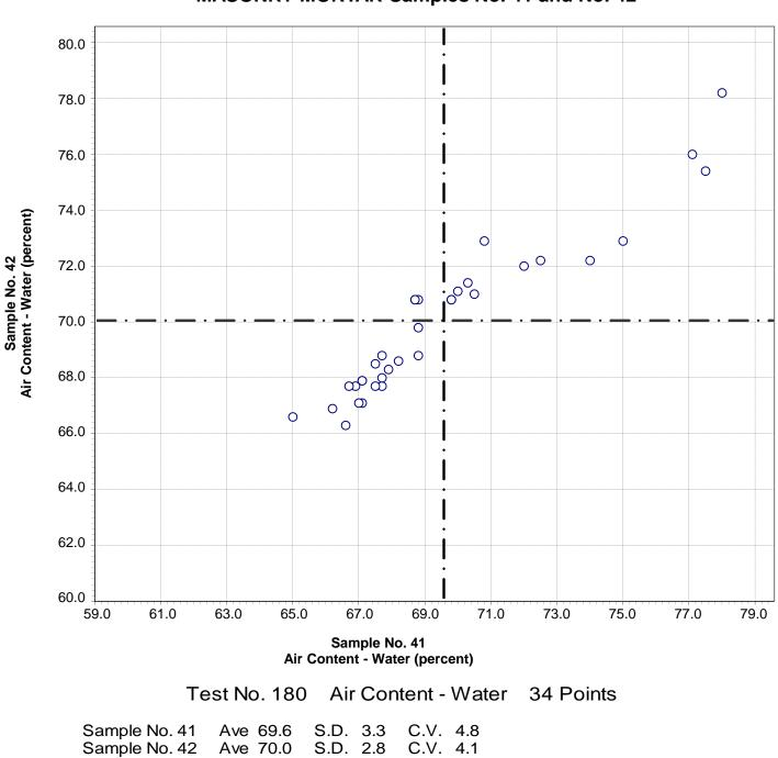
Air Content - Water MASONRY MORTAR Samples No. 41 and No. 42
