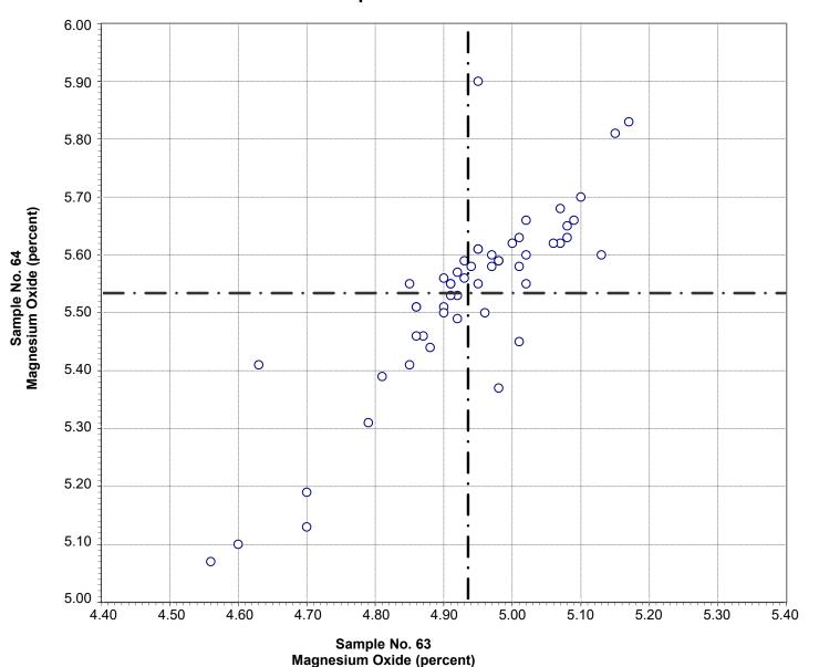
Test No. 50 Magnesium Oxide 53 Points
