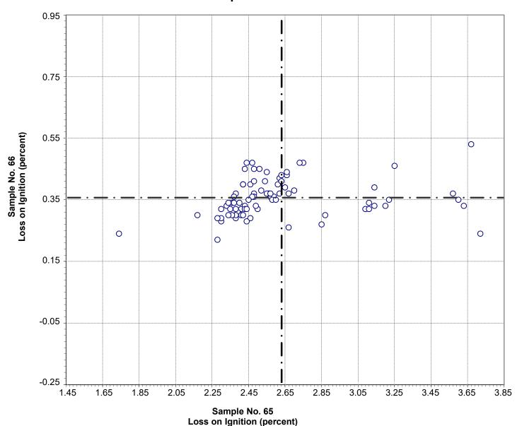
Test No. 70 Loss on Ignition 82 Points
