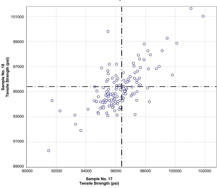
CCRL Proficiency Sample Program Tensile Strength REINFORCING BAR Samples No. 17 and No. 18
