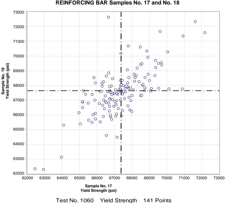
CCRL Proficiency Sample Program Yield Strength REINFORCING BAR Samples No. 17 and No. 18
