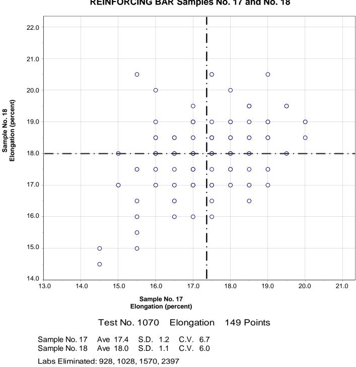
CCRL Proficiency Sample Program Elongation REINFORCING BAR Samples No. 17 and No. 18
