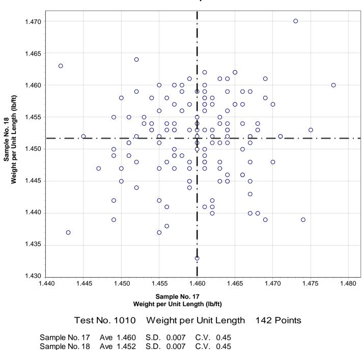
CCRL Proficiency Sample Program Weight per Unit Length REINFORCING BAR Samples No. 17 and No. 18
