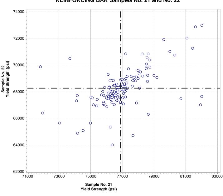
CCRL Proficiency Sample Program Yield Strength REINFORCING BAR Samples No. 21 and No. 22
