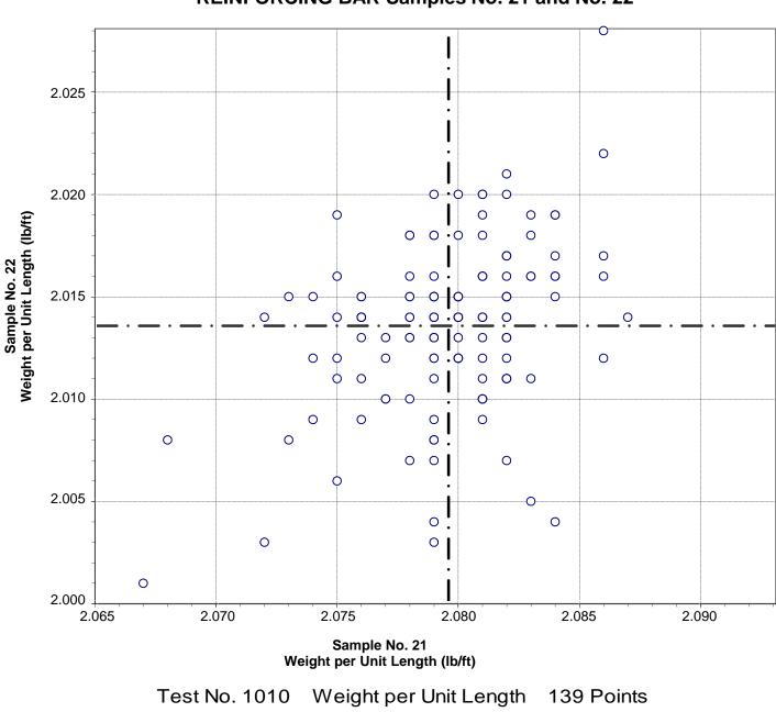
CCRL Proficiency Sample Program Weight per Unit Length REINFORCING BAR Samples No. 21 and No. 22
