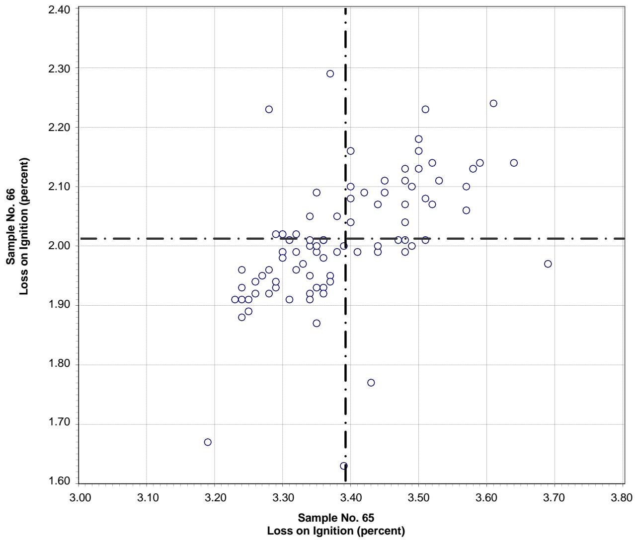
Test No. 70      Loss on Ignition      86 Points
