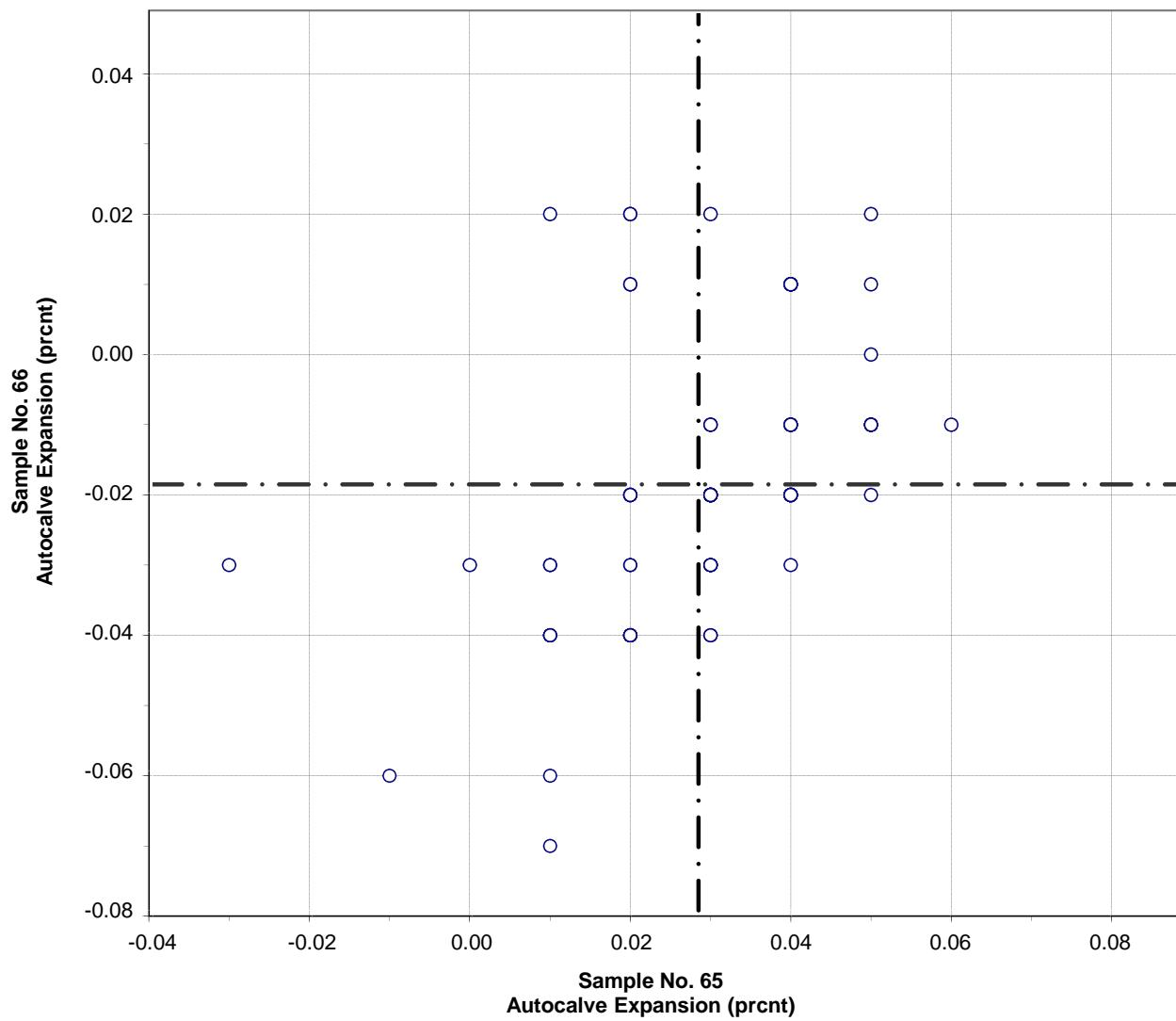
Test No. 160      Autoclave Expansion      80 Points
