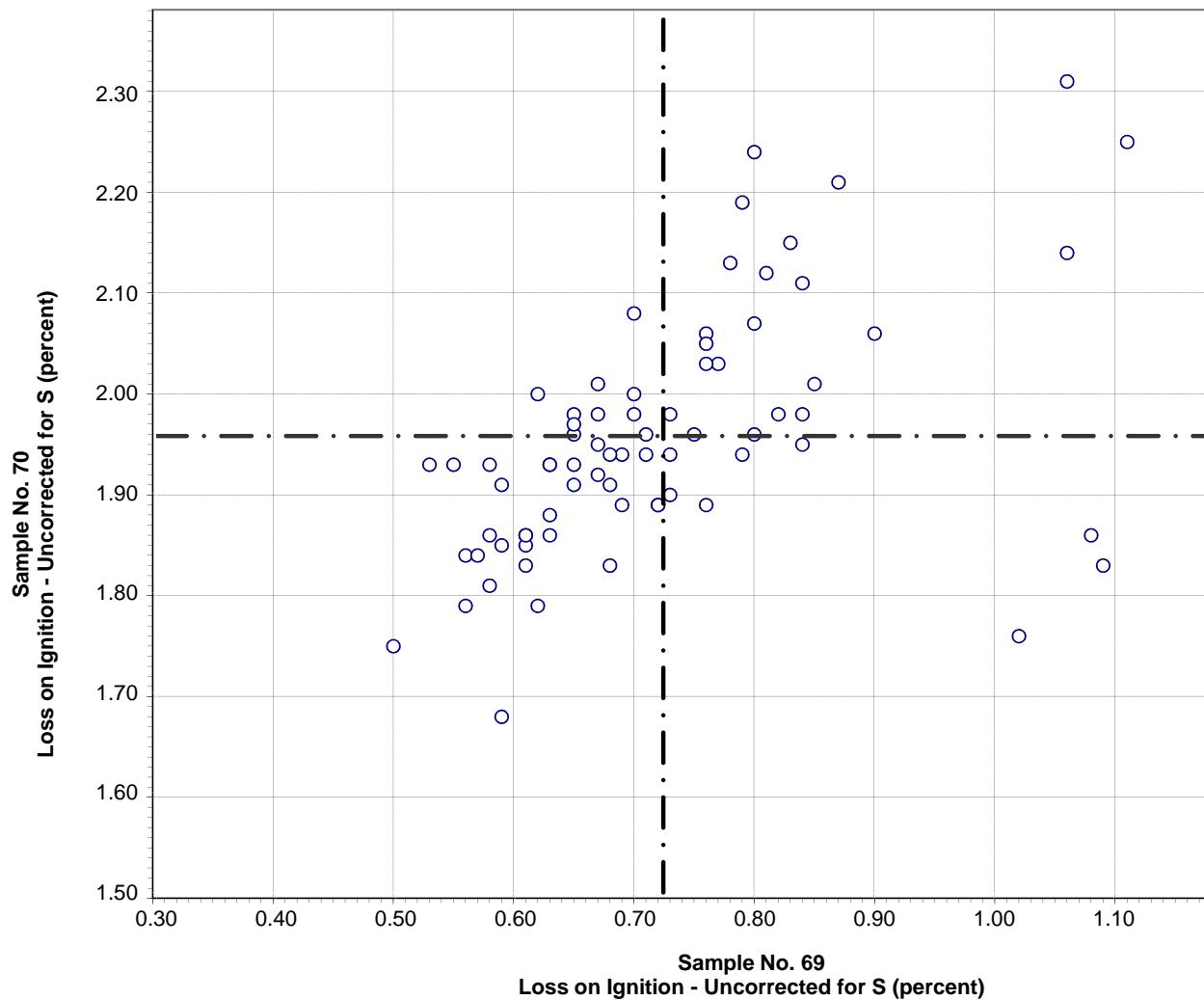
Test No. 72      Loss on Ignition - Uncorrected for S    73 Points
