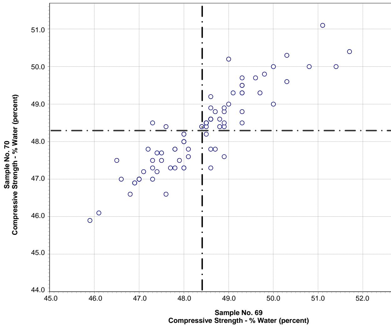
**Test No. 220      Compressive Strength - % Water    88 Points**
