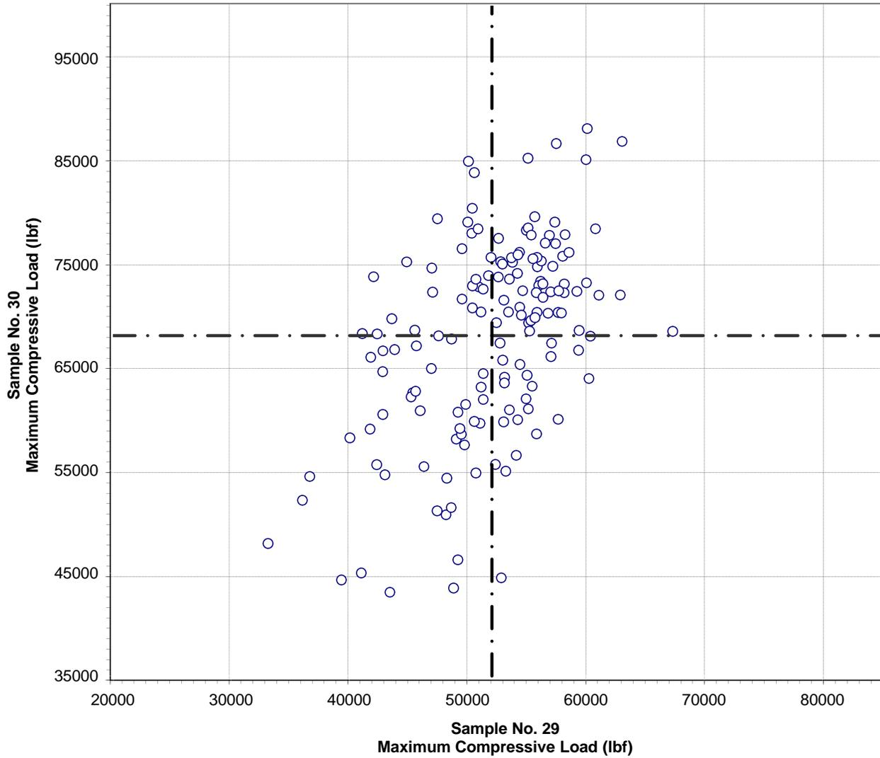
**Test No. 550      Maximum Compressive Load      151 Points**
