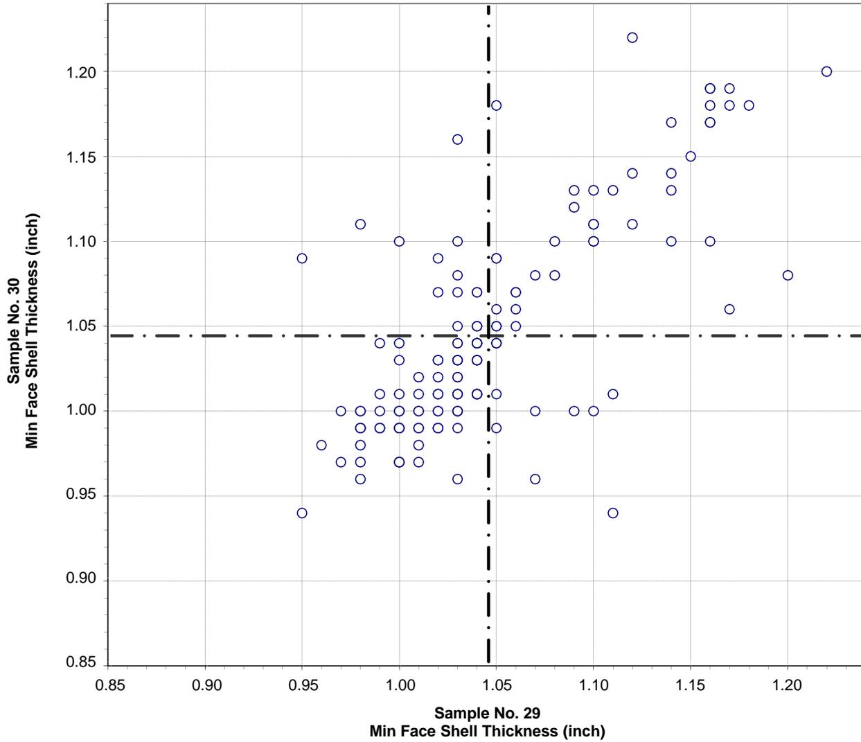
**Test No. 532      Minimum Face Shell Thickness      152 Points**
