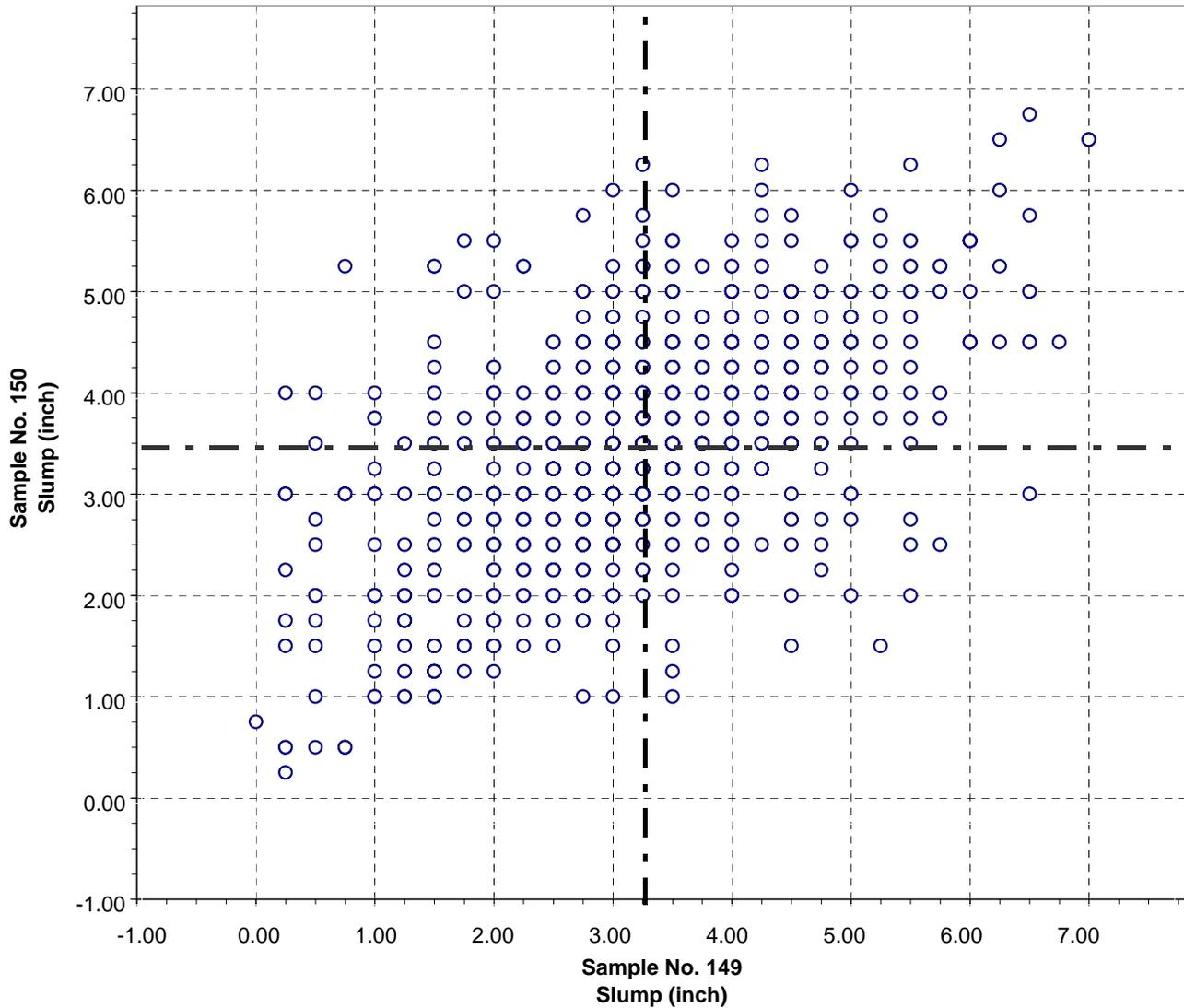
**Test No. 2      Slump of Concrete      1080 Points**
