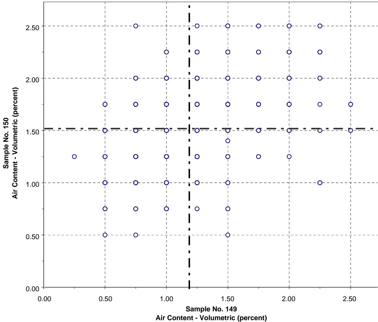
**Test No. 1      Air Content - Volumetric Method      865 Points**
