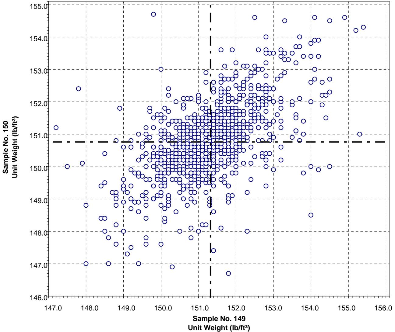
**Test No. 3      Unit Weight of Concrete      1037 Points**
