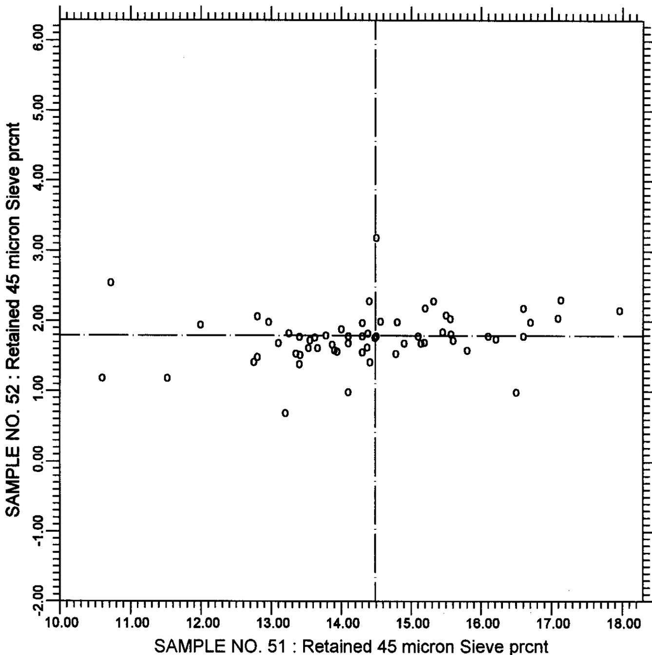
**TEST NO.281      Retained 45 micron Sieve      61 POINTS**
