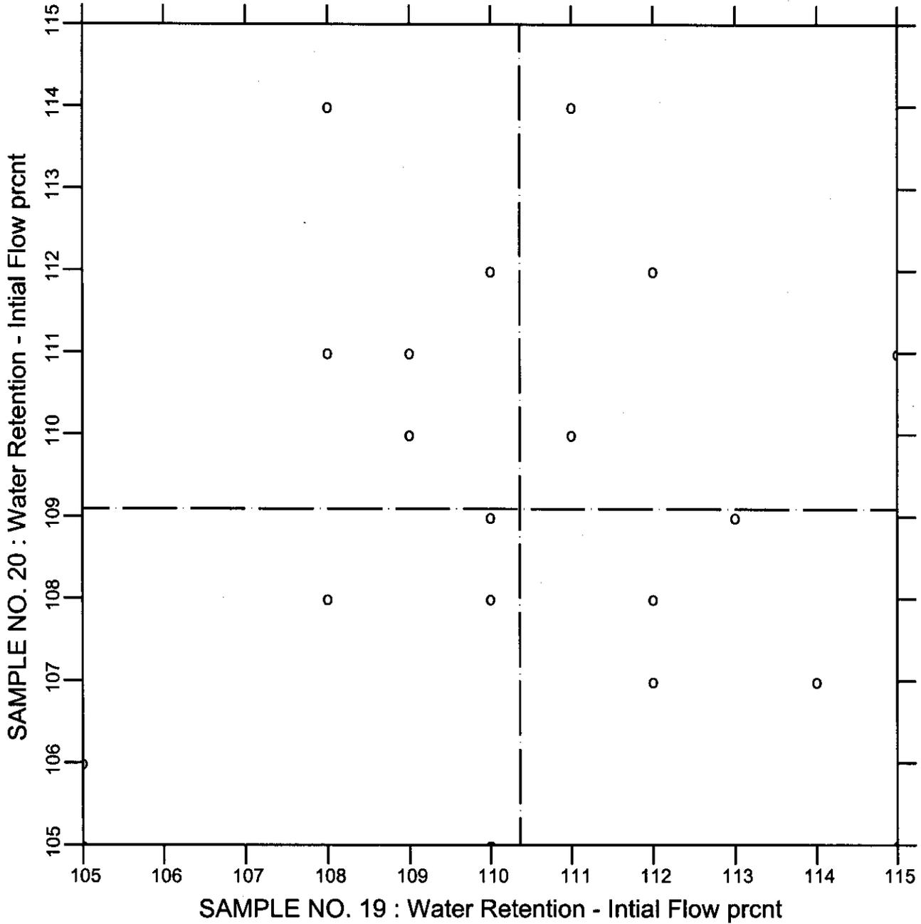
**TEST NO.331      Water Retention - Initial Flow      22 POINTS**
