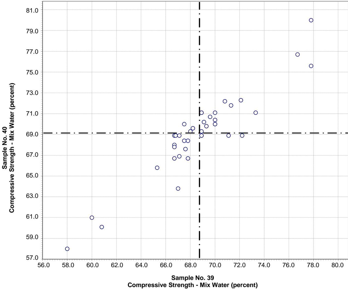
Test No. 220    Compressive Strength - Mix Water    40 Points
