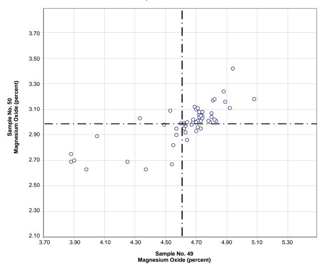
Test No. 50 Magnesium Oxide 56 Points
