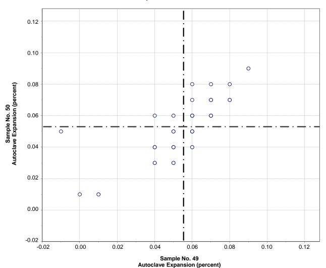
Test No. 160 Autoclave Expansion 55 Points
