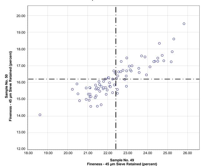
Test No. 281 Fineness - 45 µm Sieve Retained 79 Points
