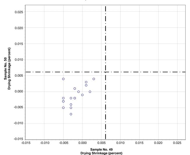
Test No. 340 Drying Shrinkage 18 Points
