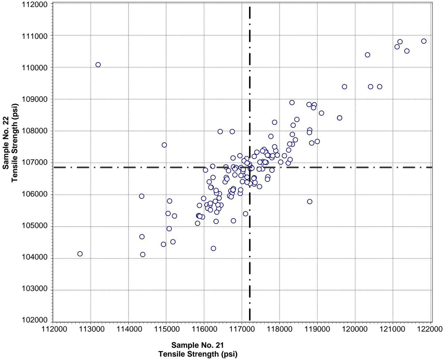
**Test No. 1050    Tensile Strength    142 Points**
